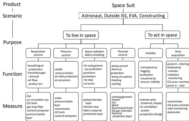
Fig. 3. Technology element decomposition in the example of space suit
