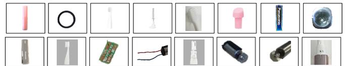
Fig. 14. Decomposition of physical product (Panasonic electric toothbrush)[8]
