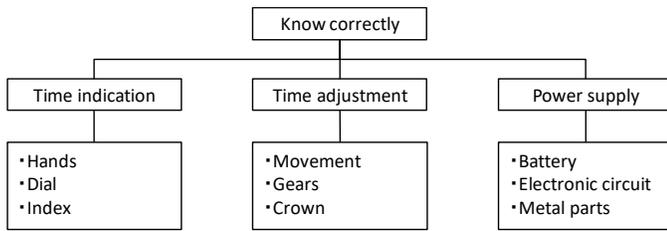
Fig. 6. An example of function-level decomposition
