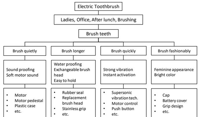
Fig. 13. Original decomposition results for an electric toothbrush
