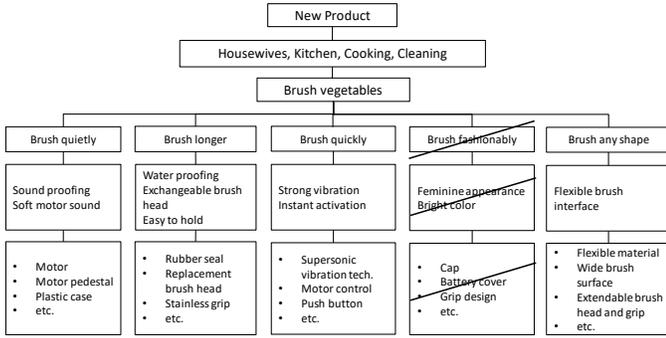
Fig. 15. Reconfigured diagram for new product based on an electric toothbrush
