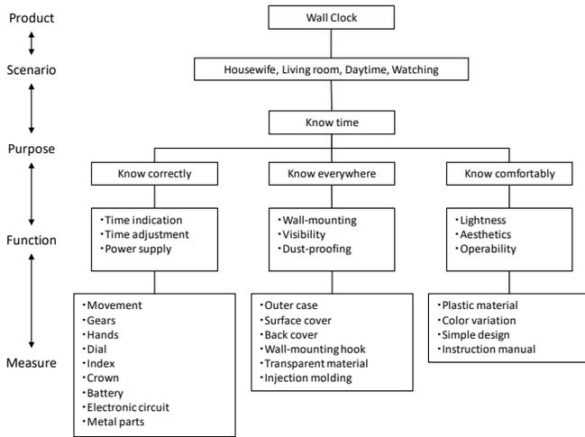
Fig. 8. An example of the technology element decomposition method applied to a wall clock
